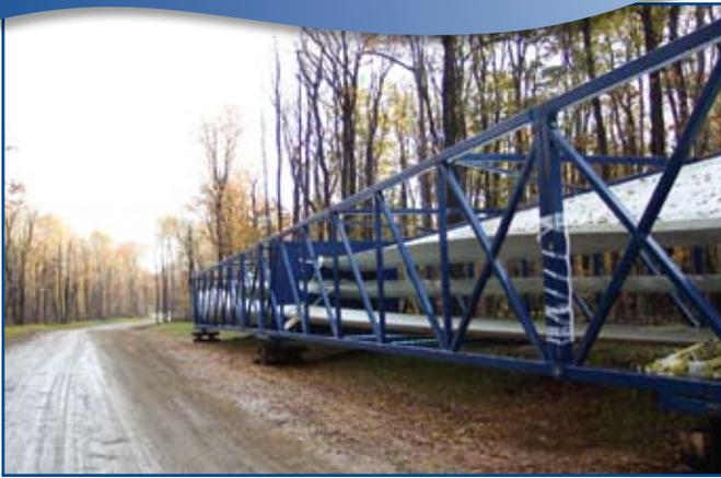
**The road to Pennsylvania's Allegheny Ridge Wind Farm site needed to accommodate large tractor-trailers used to transport the wind turbines and blades to the individual positions as well as the cranes used to erect the towers and blades.**
