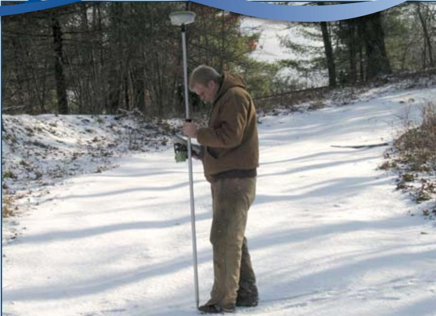
Surveyors rely on versatile tools, including this Leica System 1200 GPS-driven survey system, to gather existing topographic data in the snow-covered Pennsylvania hills.
